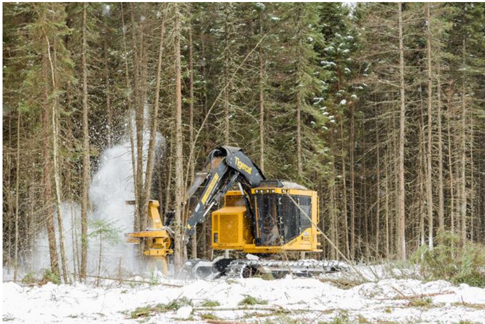
Feller Buncher removes Black Spruce gathering up to ten trees at a time.
