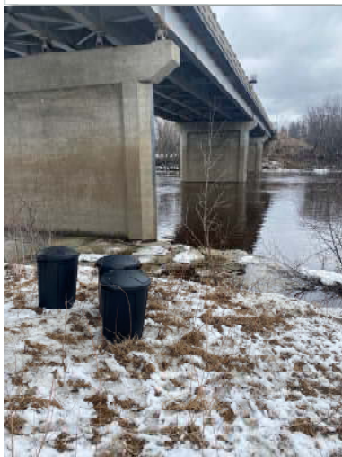
These bins are used to collect spring melt sediment samples from the Little Fork River at the bridge in Littlefork.
