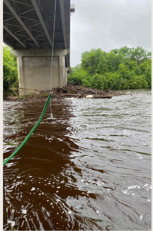
A water pump is prepared to drop into the Little Fork River for sampling.
